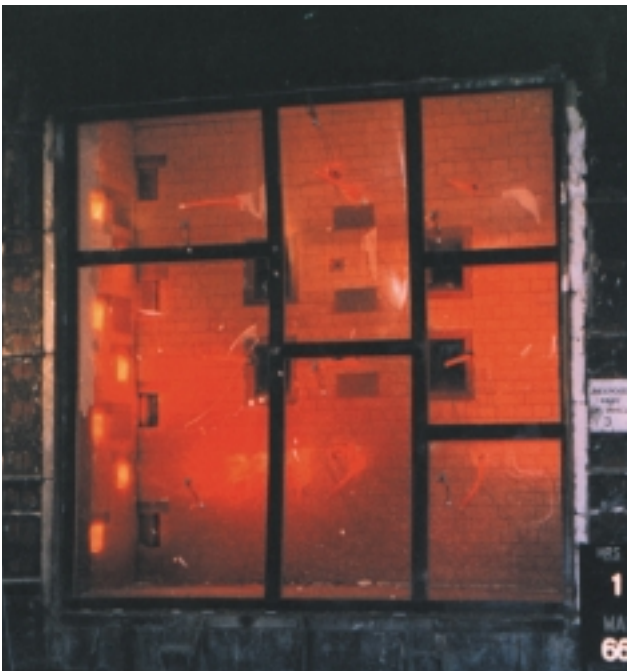
TempaFLAM Fire Resisting Safety Glass undergoing fire integrity rating test at Warrington Fire Research Institute.
